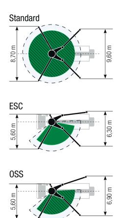
Support width based on center of support leg
