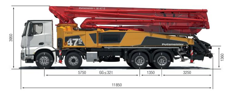
Note: Standard version. Dimensions and weights depend on truck, pump model and equipment. Dimensions in mm, MB-Arocs 4143 as example.
